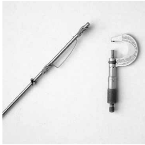
Figure 16 – Changeable spring clip pops off like a safety pin. Useable in tube ID's and sufficiently large holes in sheet metal parts.
