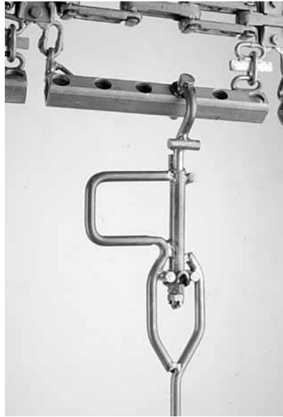
Figure 9 – Two-position detented rotator. Bend angle of hardened washer between pins determines self-locking capability.
