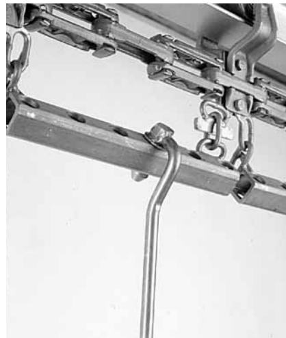
Figure 2 – Single rack top going into X-348 load bar. Yaw angle is in proportion to pin axis angle down from horizontal.
