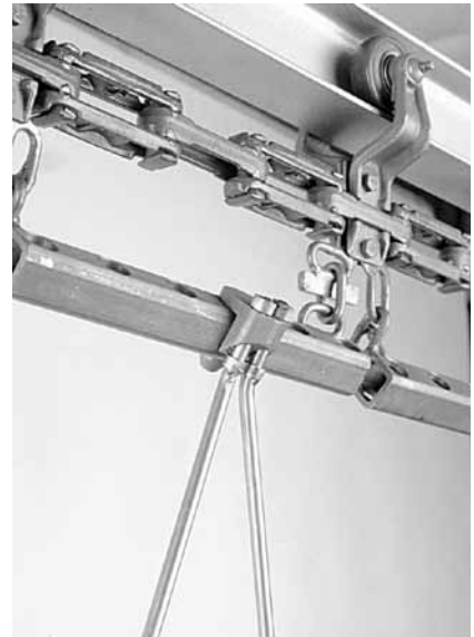
Figure 4 – Top end of eyebar rack. Rods rotate in holes in alloy steel bar engagement fitting.
