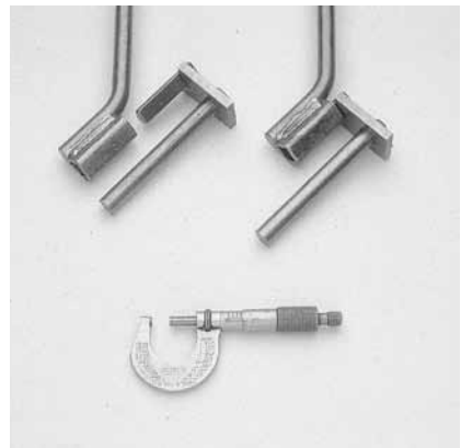
Figure 13 – Quick-disconnect joint for spray zone application. Easily disassembled after multiple coats of paint.
