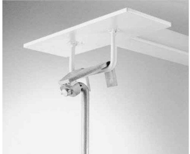
Figure 14 – Discrete devices built integral with the rack top for use on power and free systems.
