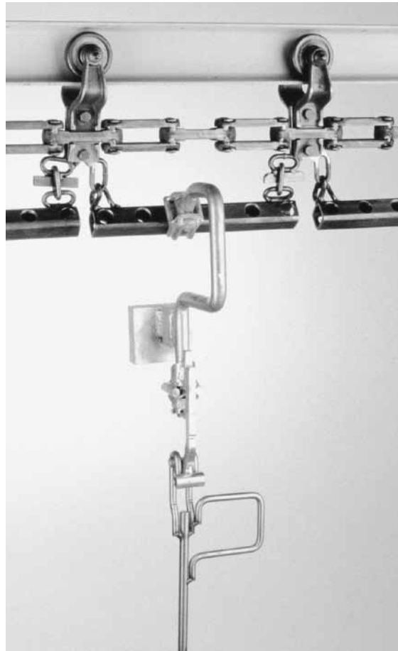
Figure 8 – C-hooks are custom designed for each system.
