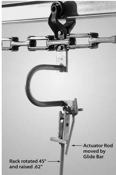
Figure 14 – Angle Pivot™ 45° Indexer in actuated position
