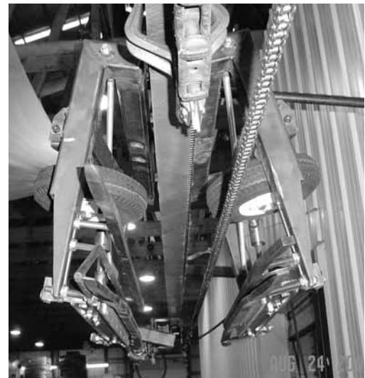
Figure 22 – Actuator Track Assembly in retracted position
