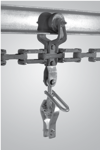
Figure 9 – Manual 180° Rotator with gravity latch. Glide bar flanking conveyor lifts latch at unload-load areas
