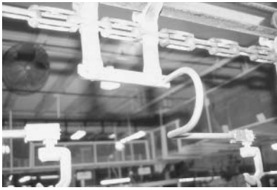
Figure 4. Corner Clear Beam with integral C-hook and rotator.
