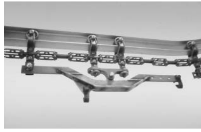
Figure 5. Corner Clear Beam with load bar rear mounting. Rear hook used for maximum line weight density; front hook for maximum weight capacity.
