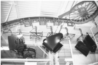
Figure 7. Corner Clear Beams of graduated lengths give non-integral trolley spacing capability.
