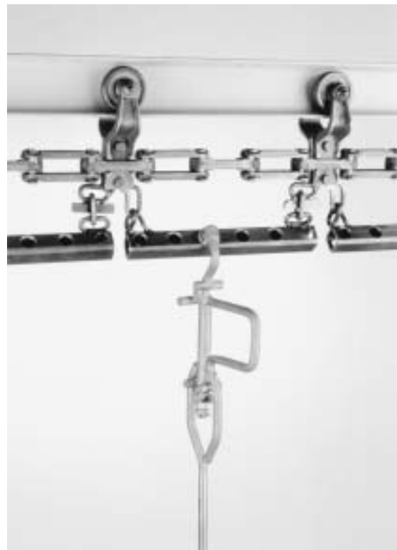
Figure 9. Positive lock rotators are double-detent devices that may be turned (manually or automatically) to facilitate loading and unloading.
