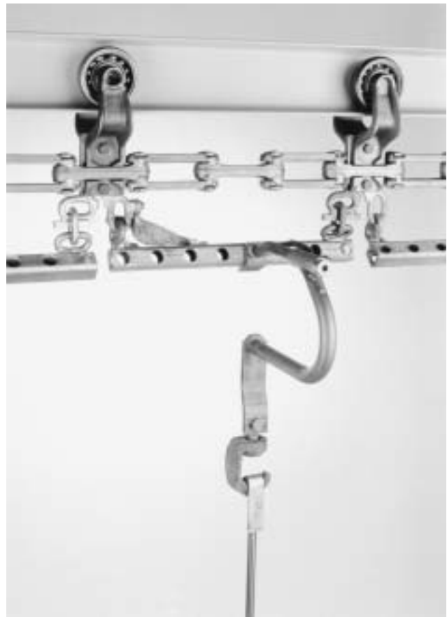
Figure 11. Ground-braid-equipped load bars and integral bearing C-hooks for nonyawing service in E-coat systems.
