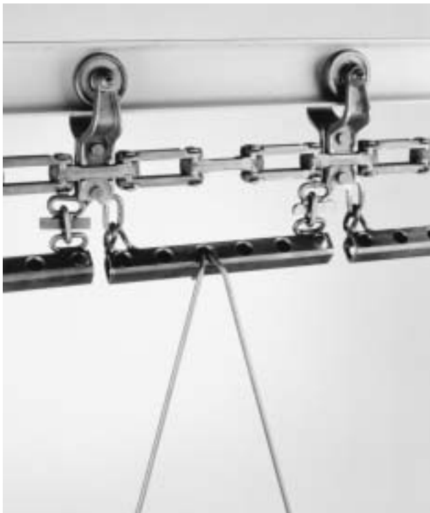
Figure 13. Paired J-hooks with pivot angle built into top, mounted in the same hole on continuous load bar systems.
