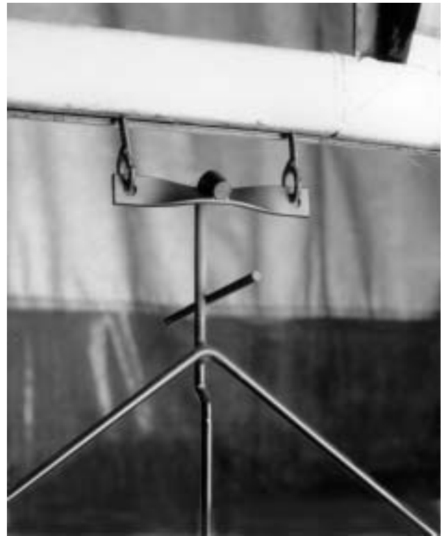
Figure 4. Basic: A load bar between two hang points on the conveyor chain, with a single payload mount bearing in the center.
