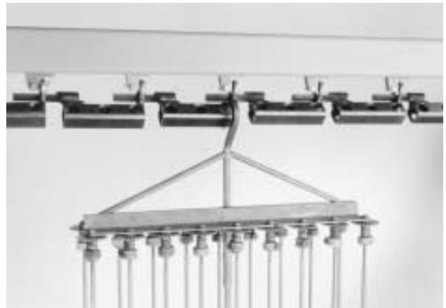
Figure 15. Power rotators for small round parts, built into the proper configuration for angle pivot use.
