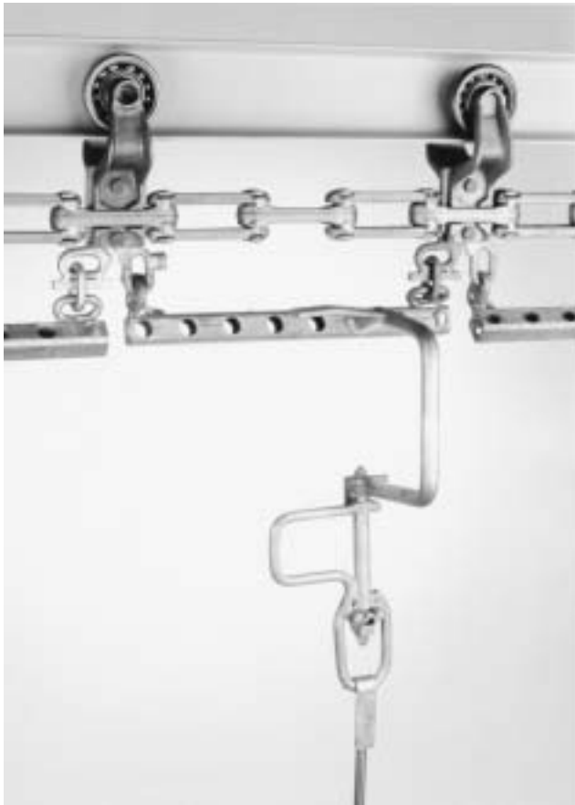
Figure 10. Rotation-stop equipped load bars for use with non-counterweighted C-hooks.
