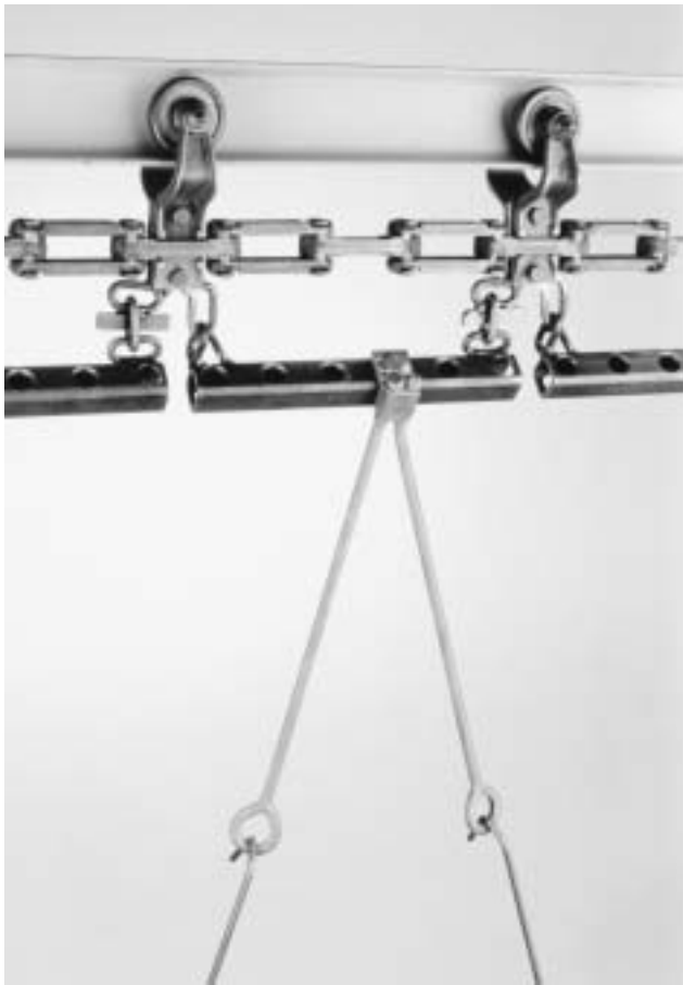
Figure 12. Eye bar tools for flat parts of varying widths on continuous load bar systems.
