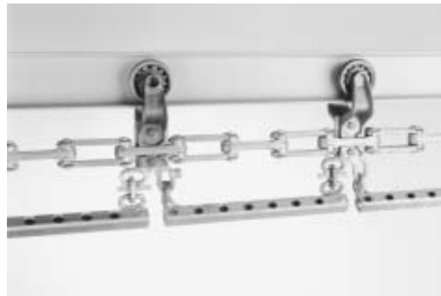
Figure 7. Continuous load bar: A more general purpose adaptation of the versions shown in Figs. 4 and 5.
